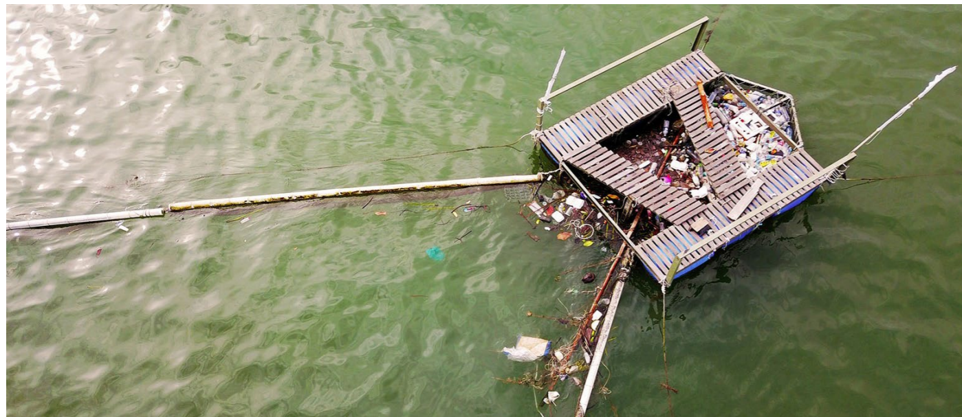
Figure 35: Litter Trap implemented in Sandakan, Malaysia
